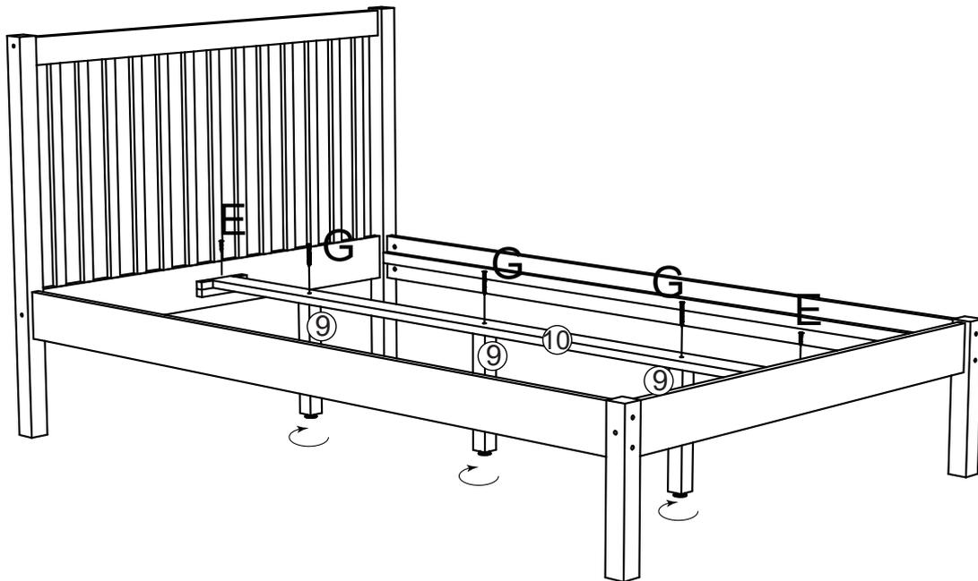
Step 5: Fix the slats(8)to the side rails(5)using hardware E with screwdriver(not provided).
