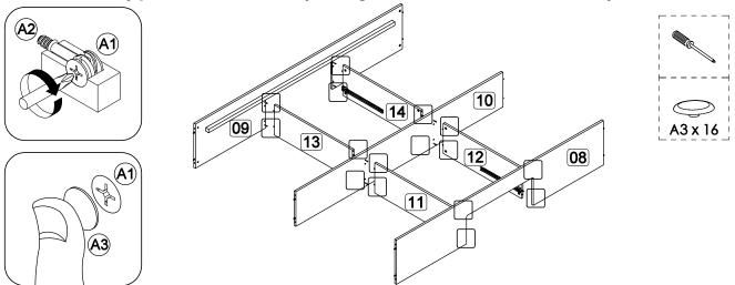
**Step 6:** Attach bed side panel (8), (9) and center panel (10) to tailstock panel (2) using hardware A1 and A2 with a screwdriver (not provided).
