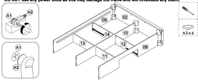
Step 7: Attach headboard panel (1) to bed side panel (8), (9) and center panel (10) using hardware C, G and H. DO NOT use any power tools as this may damage the frame and will invalidate any claim.
