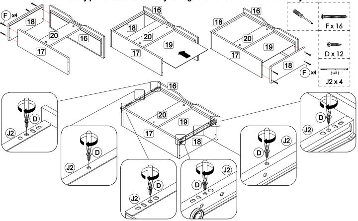
Step 11: Assemble the drawer in place along the drawer slides.
