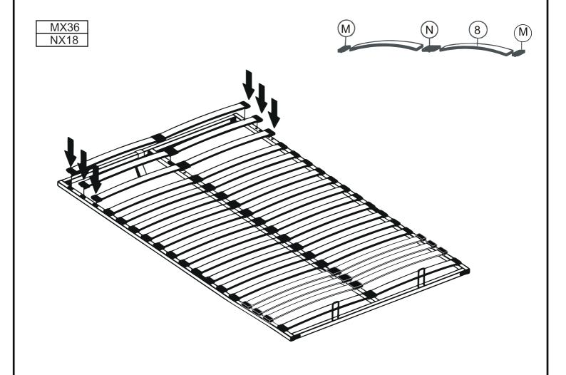
Step 14: Assemble the bed base on the right & left hydraulic frame starting from 1'to 3'as shown with HardwareH,X,R&W,and fix the support leg (16) to the bed base by Hardware G,X&R as shown.
