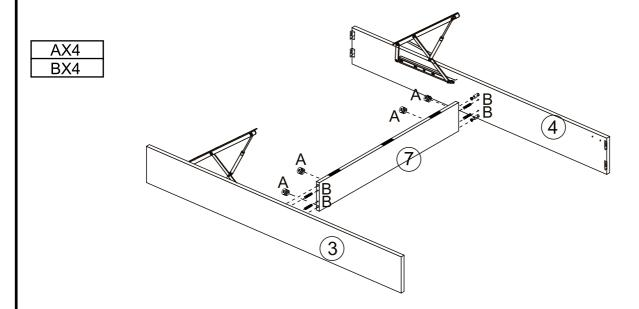
Step 10: Fix the Headboard frame and Footboard frame with the bed frame by Hardware(G).
