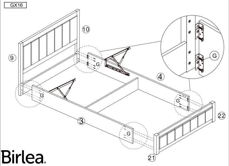
Step 11: Fix the Metal Corner Block(C) by Hardware(G).
