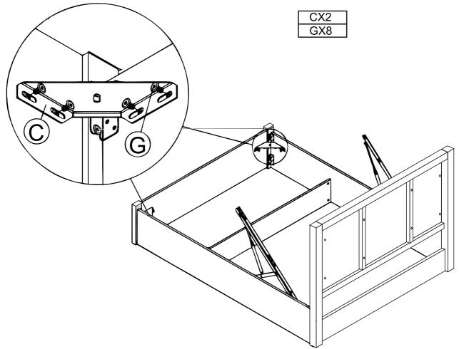
Step 12: Join together all the bed base parts (11),(12),(13) and (14) using hardware parts Q,S,X & R and also slide part P onto Part 14 before bolting together. Attach the centre rail(15) with Metal Frame by hardware G,X&R.And then attach hardware parts J as shown.
